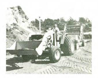
mesh and three curtain-like adjustable brushes to slow the movement of sand and debris transports refuse from the beach into the waste receptacle at the rear. This receptacle holds one and one-half cubic yards (two tons) and can be hydraulically lifted to a height of seven feet for dumping; its lid can be closed and the tilt controlled from the operator's seat. This machine cleans a six-foot swath of beach at a speed of 5.9 mph, or 3-1/2 acres of beach per hour, with only one operator.
