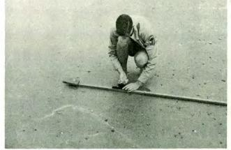
Measuring slope of sand with staff and Abney level. ↓
